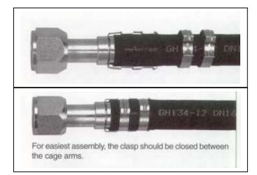
Step 6. Slide the clips over the cage arms and into the channels on each arm.
